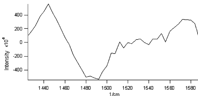
Figure 4. Transient IR spectrum produced upon excitation (266 nm) of 2,6-difluorophenyl azide (7 mM) in CD 3 CN at 273 K. The new signal at 1444 cm -1 is attributed to the triplet nitrene ( 3 N). The spectrum was recorded 0.7 μs after the laser pulse.
